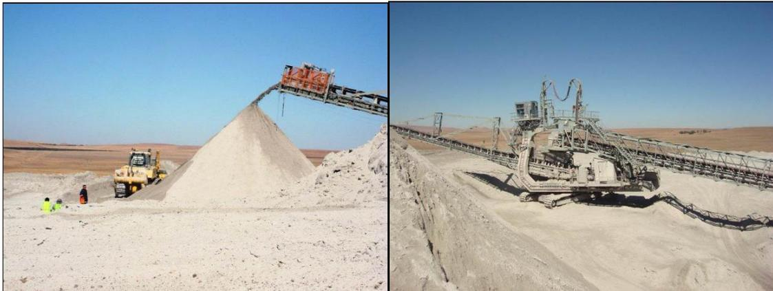
**Figure 7.1:** Stacker being used to dispose of ash at the Majuba Power Station
